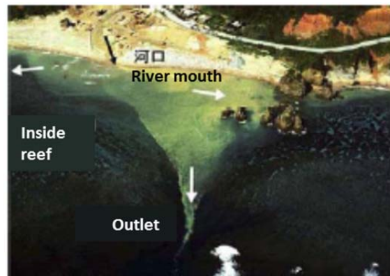
Red soil runoff spread into the sea and settle. (Sediment is partially flowing out from outlet.)
