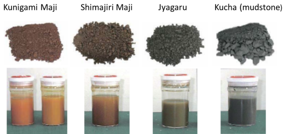
When placed into water, fine particles of soil dissolve into water, inducing turbidity.
